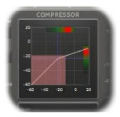
This display show the current gain transfer curve (white line), current threshold value (blue line), maximum main signal level (red area) and current main signal level (light red area).
