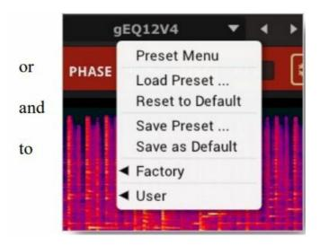
Preset menu loads and saves user presets. Presets stored under %localappdata%/gEQ12 (Windows) /Users/xxx/Library/Application Support/ gEQ12 (Mac OSX) are imported as user presets. Previous next button step trough all presets. "Reset to default" sets the current plugins settings the default settings. "Save as Default" sets the current settings as start-up/default settings. gEQ12 comes with several factory presets demonstrating the capabilities of the plugin.
