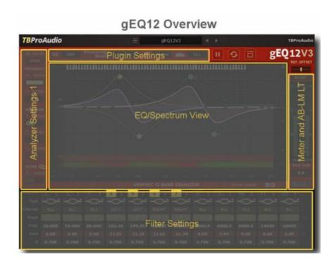
In the middle, you find the main EQ/spectrum display which lets you monitor the incoming and outgoing spectrum and adjust the filter response curve. On the bottom, you find all control of the 12 filter (e.g. type, slope and gain). On the left side the controls for the spectrum and EQ view are placed. Meters and AB-LM for perceptual loudness matching are on the right side. The top area offers plugin settings like over sampling, processing mode, phase mode and main analyzer display mode.
