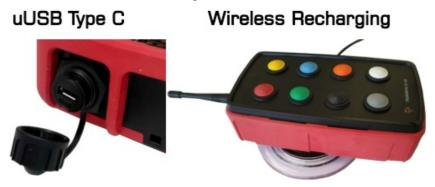
When Charging the Battery RED LED gives a slow Flash indicates charging is in progress. When fully charged the GREEN LED is illuminated
