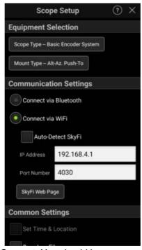
8. Return to the home screen and press Connect. You should hear a sound and a round telescope position indicator will appear on the screen. The connection will also be signaled by the appropriate diode on the box.
