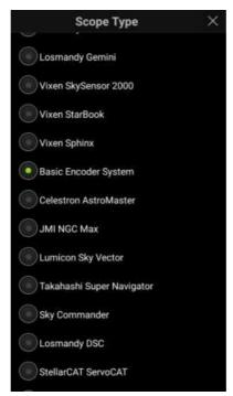
5. In the Mount Type, select Alt-Az. Push-To and enter the resolution of the encoders: 8192
