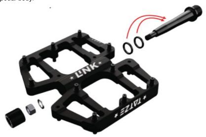
2.4. Insert nut and apply washer with a little grease. Then tighten with hexagon and Allen key in opposite direction with approx. 10 Nm.
