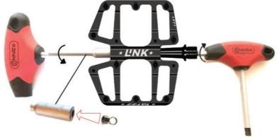
2.5 Screw in the end cap with an Allen key and approx. 10 Nm on aluminum pedals and 2.5 Nm on composite pedals. Hold the pedal while doing so.
