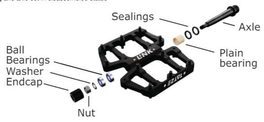
2.1. Carefully tap out the ball bearing and then clean the socket properly.
