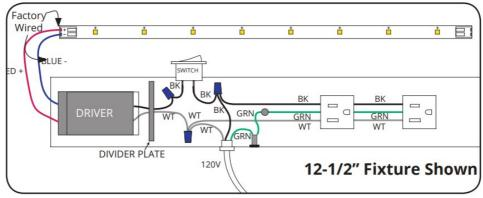
**Step 1** Secure LPS to wall by screwing into wall studs or use anchors provided. Connect BLACK Romex wire to BLACK wire from receptacles and switch.
