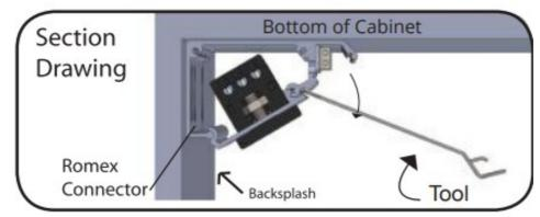
Turn power off at panel. Carefully pry open each piece with tool (provided). Insert Romex connector into knockout hole inside of back frame. Pull wires into LPS.
