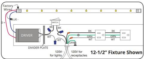
**Step 1** Secure LPS to wall by screwing into wall studs or use anchors provided. If running two circuits, one for receptacles, one for lighting, connect fixture wires to appropriate Romex wires. BLACK to BLACK. WHITE to WHITE. Ground all GREEN wires to PEM studs inside of back frame.
