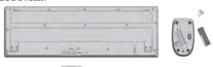
2. Insert the bundled USB dongle into your computer's USB port. It takes about ten seconds for the system to automatically connect to your wireless keyboard and mouse.
