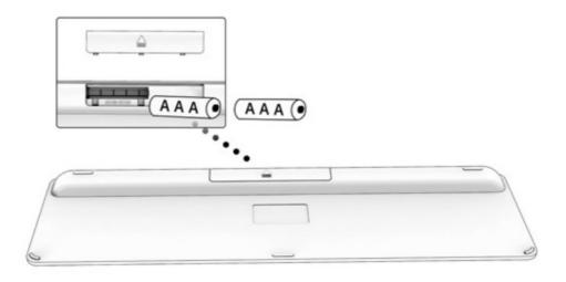
When the battery is low, the low power indicator light on the top right corner of the keyboard will flash to indicate the batteries need to be replaced.
