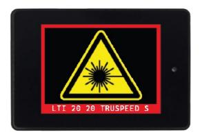
Laser protection is active for the programmed duration and then stops automatically. Laser protection can be paused at any time by tapping briefly on the screen. The system enters Cooldown.
