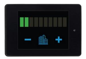
Tap twice on the right side of the screen: the display returns to the detection view. The set threshold value is displayed.
