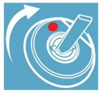
**WARNING:** If the cylinder is opened, pls pay attention to lock it again by turning it to the red dot position by the direction of the arrow (Any tool which can be inserted in the cylinder is OK)
