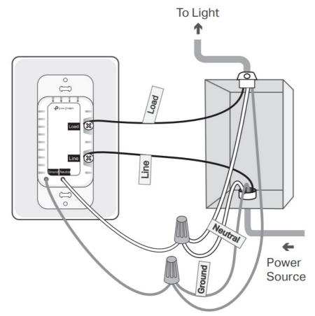
5. Line up the switch with the mounting holes. Secure it with screws.
