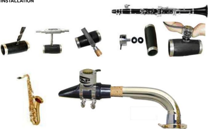
Drill hole 5.2mm on the barrel. Make the threading with {M6} hand tap cutting tool. Finish the edges of the hole with rasp. Screw the Adapter into the threading. Put the rubber ring on the Mic-sensor. Screw with care the Mic-sensor into the adaptor. Twist the cable on the barrel for protection.
