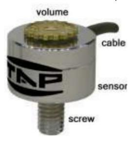
Drill hole 5.2mm on the barrel. Make the threading with {M6} hand tap cutting tool. Finish the edges of the hole with rasp. Screw the Adapter into the threading. Put the rubber ring on the Mic-sensor. Screw with care the Mic-sensor into the adaptor. Twist the cable on the barrel for protection.
