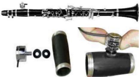
Drill hole 5.2mm on the barrel. Make the threading with {M6} hand tap cutting tool. Finish the edges of the hole with rasp. Screw the Adapter into the threading. Put the rubber ring on the Mic sensor. Screw with care the Mic-sensor into the adaptor. Twist the cable on the barrel for protection.
