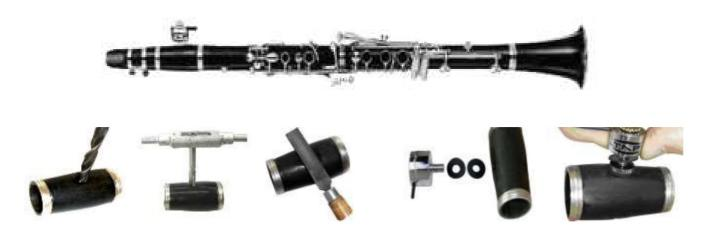
\*\*\* Drill hole 5.2mm on the barrel. Make the threading with {M6} hand tap cutting tool. Finish the edges of the hole with rasp. Screw the Adapter into the threading. Put the rubber ring on the Mic-sensor. Screw with care the Mic-sensor into the adaptor. Twist the cable on the barrel for protection.
