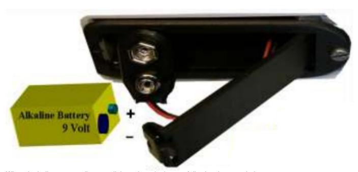
When the indicator goes dim or no light replace the battery following the steps below:
