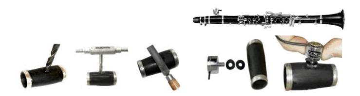
\*\*\* Drill hole 5.2mm on the barrel. Make the threading with {M6} hand tap cutting tool. Finish the edges of the hole with rasp. Screw the Adapter into the threading. Put the rubber ring on the Mic-sensor. Screw with care the Mic-sensor into the adaptor. Twist the cable on the barrel for protection.
