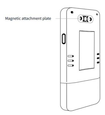
• Two 4 mm diameter screw holes allow for fixing the plate to the surface with screws (not supplied).
