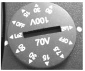
7. The CVS 8 is fitted with a 60 W transformer. When used in distributed-line systems, the transformer can be tapped at 60 W, 30 W, and 15 W, with an additional 7.5 W tapping for 70.7 V line systems.
