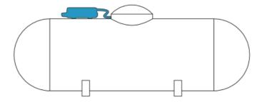
**NOTE:** Do not place the tank monitor under a steel lid or inside the collar since this can prevent the monitor from connecting to the cellular network.
