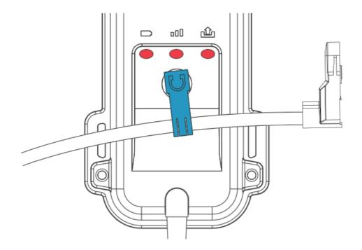
This will prevent the monitor from sending additional readings. Hold the activation magnet over the activation pad for approximately 15 seconds until all 3 LEDs are red. Remove the activation magnet while all 3 LEDs are red.
