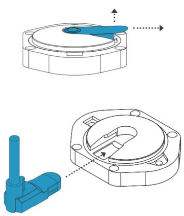
The Tank Utility remote level monitor can be installed on all tanks equipped with a Remote-Ready Dial. If your Remote-Ready Dial has a black dust cap, you will first need to remove it by simultaneously pulling up on the tab while sliding the dust cap out of the dial. If applicable, route the cable through the hole in the tank's collar or lid. Slide the sensor into the dial slot until you feel it click.
