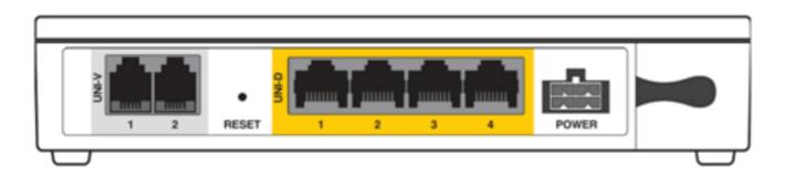
Using an Ethernet network cable, connect your router from its WAN port to the relevant Uni-D port on the NBN Connection Box. We generally activate the next available Uni-D port – starting with Uni-D 1. We will detail your Uni-D port number in our emails to you.
