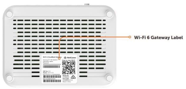
Contains your Wi-Fi network name and Wi-Fi password. You'll need these to connect your devices to Wi-Fi. **Back View of Device**
