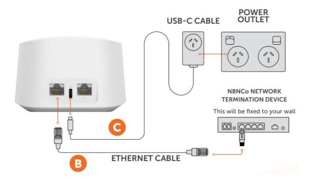
**IMPORTANT:** You will need to plug the ethernet cable from your eero 6+ into your Network Termination Device's activated Uni-D port. If you are unsure which port has been activated, check your NBN Ready to Go email from us
