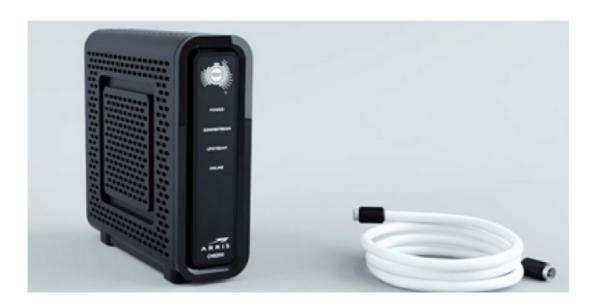
**Step 2**Ensure that this the NBN Connection Box is connected using the white HFC cable to the cable wall socket. This should have been completed during the NBN activation appointment.
