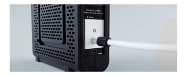
**Step 3**Ensure that power is connected to the NBN Connection Box. The POWER, DOWNSTREAM, UPSTREAM and ONLINE lights should be on.
