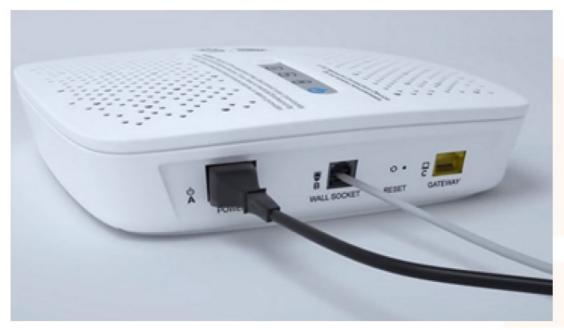
• Step 4: Connect your BYO router to the NBN Connection Device (NCD). Use the WAN port on the back of your BYO device and the Gateway port on the NBN NCD.
