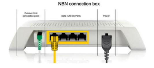
Using an ethernet network cable connect your router from its WAN port to the relevant Uni-D port on the NBN Connection Box. We generally activate the next available Uni-D port – starting with Uni-D 1.
