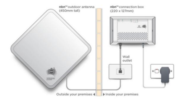
**Step 2**Ensure that the power cable is securely in place and that the POWER, STATUS and ODU lights are on and solid green. You should see at least one signal strength light on (this may be flashing).
