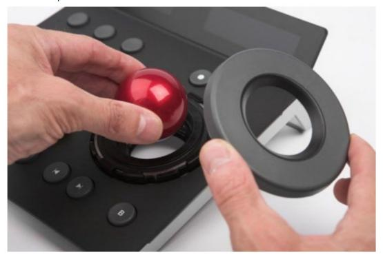
The ring on the trackerball is held in place by magnets in the ring. When replacing the ring make sure it locates correctly down on the trackerball. If it's in place correctly then there will be about a 1mm gap between the bottom of the ring and the panel surface.
