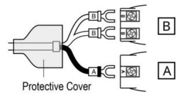
In the case of a 4-wire sensor, one of the A wires will be left disconnected.
