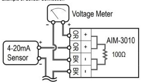
It is possible to connect a sensor and a voltage meter to the module at the same time.
