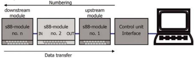
The information is transmitted from the S88-6 via the s88-bus to the upstream feedback module or to the connected digital device (interface, memory or central unit). The data transmission from one feedback module to the other takes place in the s88 bus according to the bucket-chain-memory principle. The number of feedback devices you can connect to a bus line depends on the interface, memory or central unit you use. Please observe the specifications of the device manufacturer.
