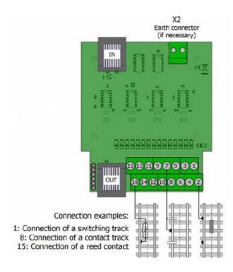
After performing a successful functional test install the S88-6 at the desired place on your model railway. Connect the inputs 1 to 16 to the mass contacts and connect the module to the central unit, the memory or the interface or to another feedback module.
