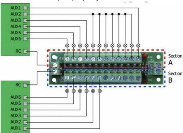
If more than 12 connections are required, the two sections can be connected by connecting the two connectors of X2. Then, however, only one circuit may be connected!
