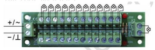
Note: When connected to DC voltage, one of the two LEDs on the board lights up to indicate on which side the positive voltage (+) is applied. When connected to AC voltage, both LEDs light up.
