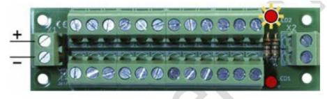
When connected to an AC voltage source, both LEDs light up.
