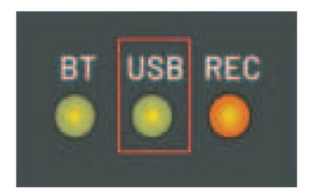
**c.** REC MODE (see picture on the right) While a USB drive is inserted via USB-A and mixer under USB playback mode (i.e., green USB indicator glows), press and hold MODE button for 3 seconds to enter REC mode. In this case, the REC indicator flashes red while recording normally. Press and hold MODE button for 3 seconds again to pause recording (REC indicator glows solid red). Again, press and hold MODE button for 3 seconds to exit REC mode and start playback of the recorded file.
