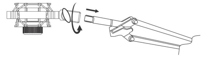
2. Align the front of the mic (marked "SM20" and polar pattern ) with the sound source, place it in the shock mount, and tighten the bottom nut securely.
