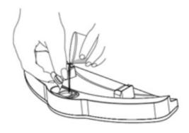
Place the bottom of the machine upward, align the positioning column of the water tank with the positioning hole of the carriage at the bottom of the machine, and press the water tank tightly.
