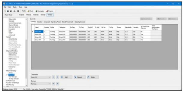
Typically the "Label" is configured to match the talkgroup name. This label will be displayed on the screen. As soon as this basic template has been programmed, the radio will hunt and attempt to acquire service on the system.
