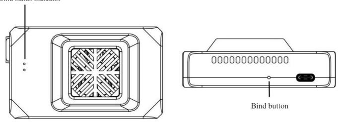
The 2 LED lights of air unit are used to indicate the bind status only, when air unit is in binding, they will be flashing in yellow/green respectively.
