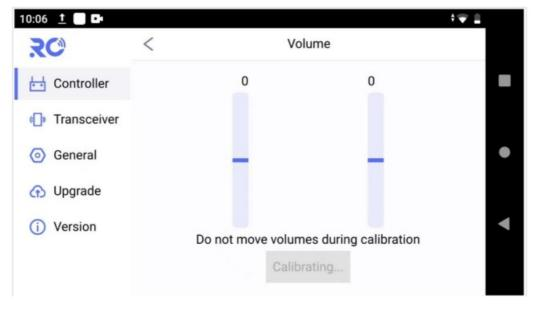
4. Go on with end point calibration. According to the prompt, move volume fully in each direction, afterwards, touch on "Complete" to finish the correction operation.
