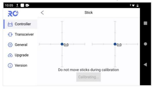
Go on with end point calibration. According to the prompt, move stick fully in each direction, afterwards, touch on "Complete" to finish the correction operation.
