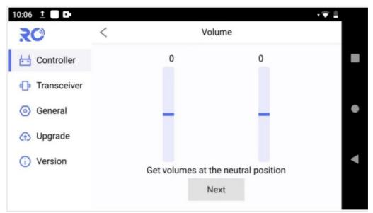
3. If the volumes stand still already, but the output value is not 0, it means the volume neutral position has an offset. Now do not move the volume, touch on "Next" to do neutral position calibration.
