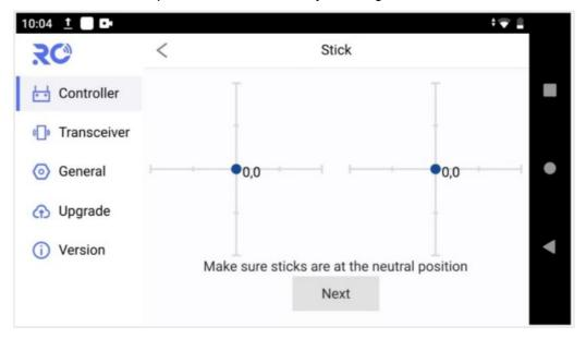
If the sticks are at the neutral position already, but the blue dots are not at the central, it means the stick neutral position has an offset. Now do not move the stick, touch on "Next" to do neutral position calibration.
