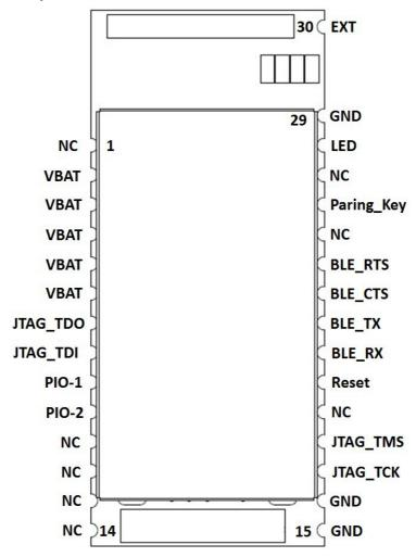
Figure 1: Pinout
