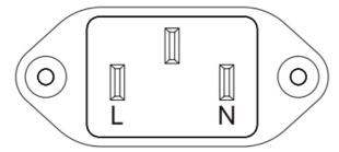
• Power Sockets – FILTERED Output (Power filter front panel facing left)
