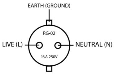
If you audio-video equipment has the phase marking for the power cable input, make sure to connect the equipment power cable plug to the filter.
