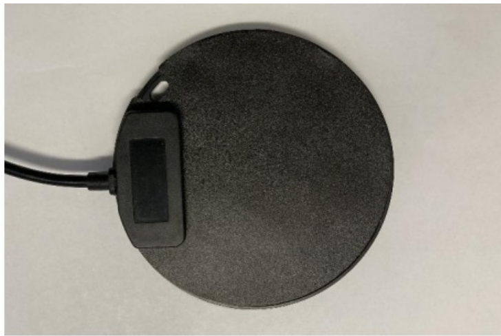
Image 4. SmartSense Tag – charging cable plugged into the charging port.
