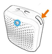
5.6. While blue LED is blinking, tap on update button to initiate firmware update for Tack GPS device.
