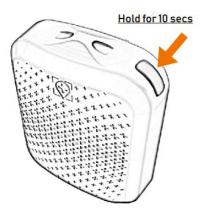
5.5. Single press on power button to power up the device again. LED will start blinking blue.
