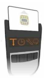
In order to enter into device setup a smart card has to be inserted into smart card slot in inverse way (chip outside).
