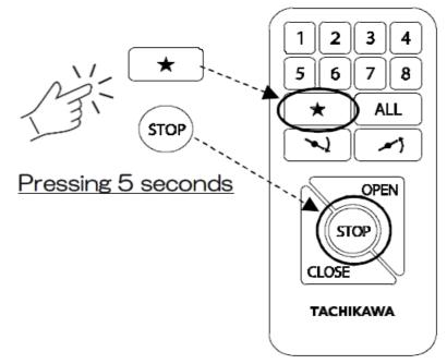
3. The blind(s) will move up/down, and a buzzer will sound when the setting is correctly completed.
