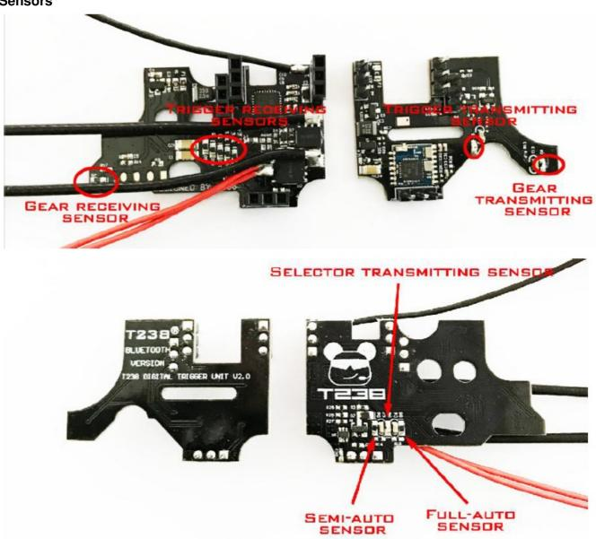
**Receiving sensors:** 5 trigger receiving sensors, 1 gear receiving sensor, 1 semi-auto sensor and 1 full-auto sensor. Transmitting sensors: 1 trigger transmitting sensor, 1 gear transmitting sensor and 1 selector transmitting
