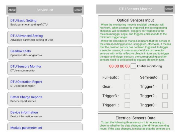
Go to "DTU Sensors Monitor", and enable the "Enable monitoring" checkbox, move the trigger, selector plate and the sector gear to see if the corresponding checkbox changes. If no, means that the corresponding position sensor is faulty or the installation is faulty, and the corresponding sensor cannot be triggered. It is suggested to open the gearbox for investigation.
