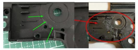
16. Check whether the top board can be leveled against the gearbox. If not, it is recommended to modify the gearbox first.
