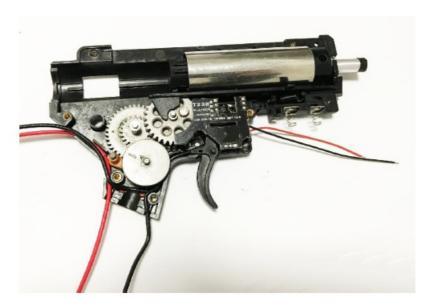
19. Clean the gearbox and gears, and use less gear oil as far as possible, so as not to pollute the sensors and affect the normal operation of DTU. After confirming that there is no problem, install the other side of the gearbox and tighten the screws.
