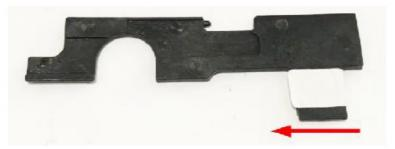
28. If you only get a SEMI-AUTO function and a FULL-AUTO function without SAFE function after the gearbox is installed into the receiver, the position of the white sticker on the selector plate should be not correct, it indicated that the semi-auto or full-auto sensor can still be activated when the selector plate is in the SAFE position. Move the white sticker to the right 1-2mm until the functions are normal.
