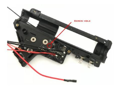
10. Check whether the components on the back of PCB will affect the installation, if so, please modify the gearbox first.
