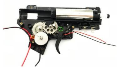
18. Insert the top board and make sure the rubber pads are relaxed. They will only be squeezed when the other side of the gearbox is installed.
