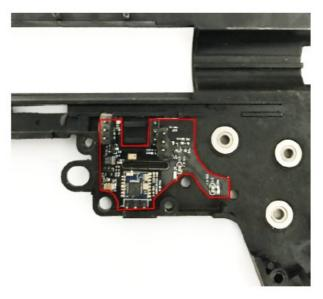
17. Put everything back into the gearbox, except 3 parts in step 8. Make sure the trigger does not touch the DTU.
