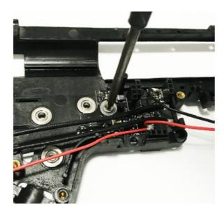
13. Adjust the wires, make sure that the sensors' surface are clean and not blocked.
