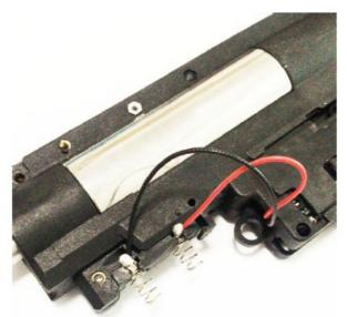
24. After correct installation, when the selector plate is in SAFE position by default setting, the trigger can still be pulled, but the DTU will not react. When the selector plate is in SEMI-AUTO or FULL-AUTO position, the DTU will react.
