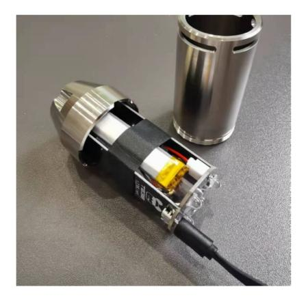
Screw off the shell and plug in the USB cable. The red LED lights up when charging and goes out when full.
