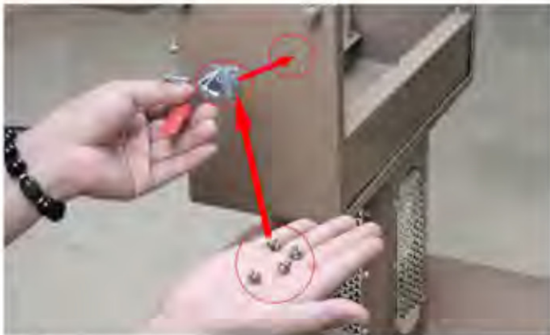
4. The chassis switch is located above. Remove the four screws on both sides of the chassis
