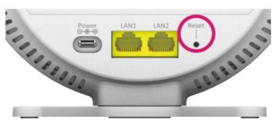
3. Withdraw the paperclip. LED on the front panel displays blinking red to indicate factory reset in progress
