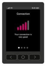
Like your phone, the gateway displays up to five bars on its Connection screen, indicating signal strength. The number of bars you see represents the strength of the gateway's current connection to the cellular network. An X indicates the gateway is not connected to the cellular network.
