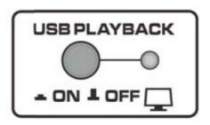
**NOTE:** When this switch is placed in (.-.),the USS playback passes through the CH5-6 output and the LED lights up
