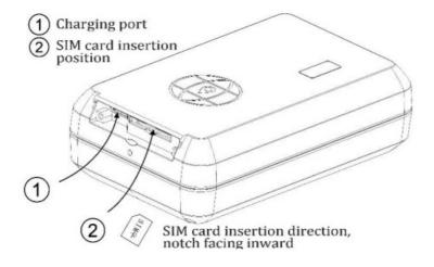
• After the SIM card is inserted, the device powers on using the backup battery. If the device fails to power on due to low battery, you can connect the device to the external power.
